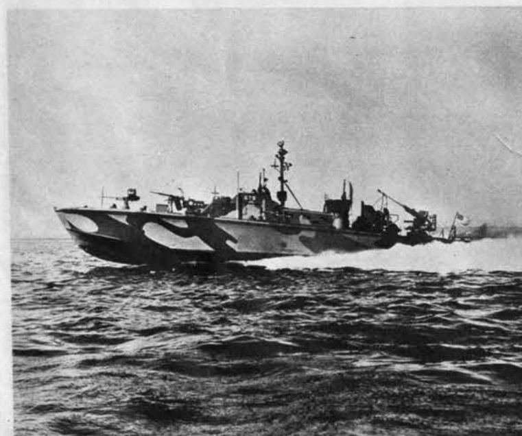
Comb-type radar on latest U. S. PT may be used widely in the future. Tougher to spot than the radome at top, it is still a recognition clue.
